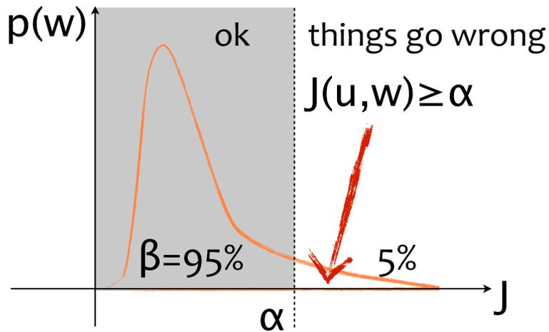
**Control objective:** minimize the **Conditional Value at Risk (CV@R)**, a risk measure of the profit that quantifies the average loss above a given threshold
